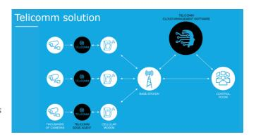
Telicomm's solution enables connecting 20-30 HD-cameras over a single cell of 4G cellular infrastructure in a robust way (compared to 2-3 cameras with current technology), answering the need of the municipalities. These numbers were validated both by extensive simulations as well as demo system.
